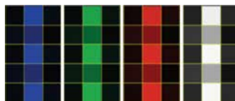
圖 3.3d: How the pixels of a sensor interpret the spot sizes in figure 3.3c.
